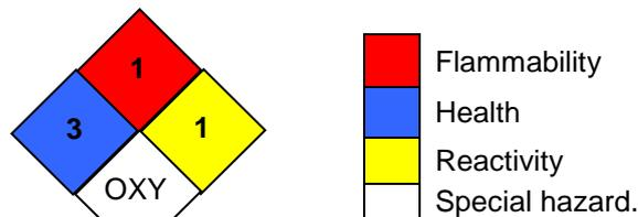
Hazard rating: 0 - Minimal; 1 - Slight; 2 - Moderate; 3 - Serious; 4 - Severe; RNP - Rating not possible
